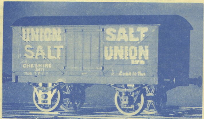
Fig. 14. Compensation action may be seen by the LH wheel mounting an obstruction. Note the method of mounting axleboxes on the projections of the CSU bearings, leaving clearance for the compensating action between the spring and axlebox mouldings.
