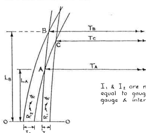
I<sub>1</sub> & I<sub>2</sub> are normally equal to gauge or gauge & interval.
